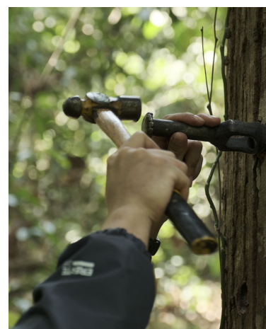
Hollow steel punch - cambium tissue
